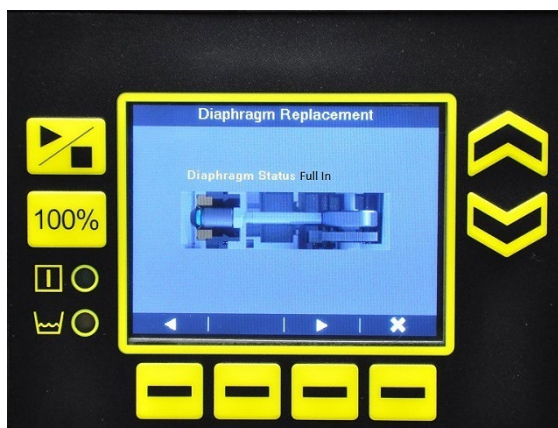
Figure 33: Diaphragm Replacement (Full In)
